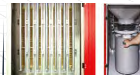
Easy access to filters and dust bins
